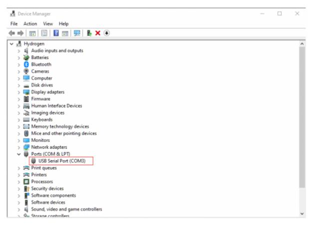
Example: On HedgiePi's computer, the OpenDMX controller is showing up on COM 3.
