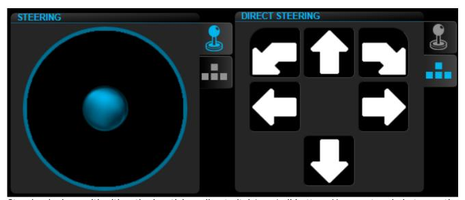
Steering is done with either the joystick or direct pitch/yaw/roll buttons You can toggle between the two with the buttons on the side of the steering component.
