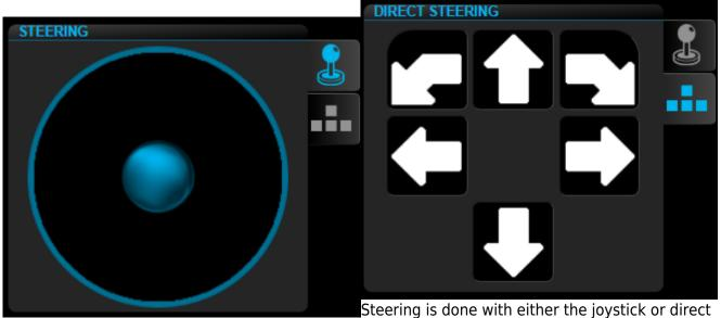
pitch/yaw/roll buttons You can toggle between the two with the buttons on the side of the steering component.
